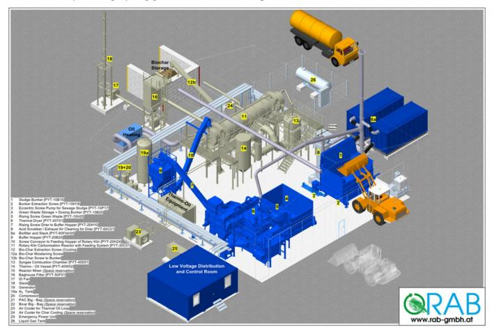
*Figure 2:* HSY's sludge pyrolysis pilot plant and the steps of sludge-char production in the unit, described in short below as presented by HSY's R&D portfolio manager and HSY's official website (HSY, 2021b)
